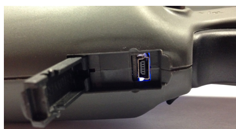
Mini USB port for programming with SP-18V-V2 programmer
