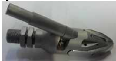
Nozzle version automation with non return device
