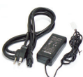
AC Adapter AD-24-IT19 ● EDP No. 806081 AD24-IT19E ● EDP No. 806137 Use with IPC-A4, IPC-A3 I/P : AC100V~240V 1.2A O/P : DC24V 1.9A
