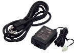
AC Adapter AD24-IT ● EDP No. 806051 AD24-ITE ● EDP No. 806135 I/P : AC100V~240V 0.4A O/P : DC24V 0.75A
