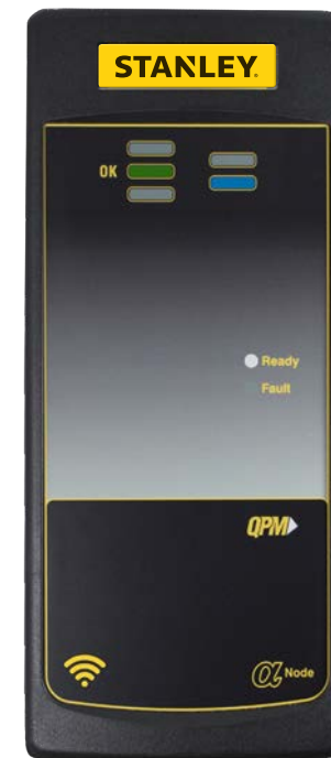
QB0301 IEEE 802.15.4 Can manage One STANLEY Cordless Tool
